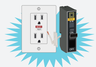
A listed outlet branch-circuit-type AFCI receptacle in combination with a listed branch-circuit overcurrent device
