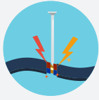
Wiring damaged by screws or nails
